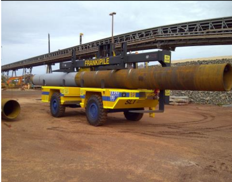
Testing of side-loaders for Wheatstone, Australia
